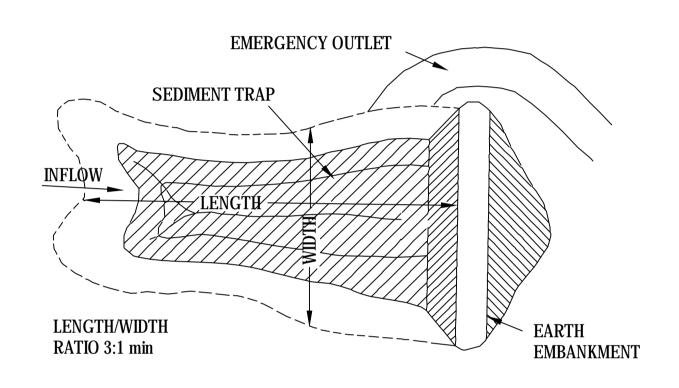
PLAN VIEW OF TYPICAL SEDIMENT BASIN NTS
