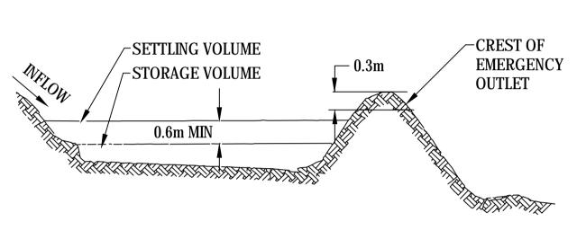
CROSS SECTION OF TYPICAL SEDIMENT BASIN
